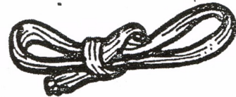
Hank – If rope is put away untidily, it will tangle and fray. The hank is a simple way to store ropes neatly.
